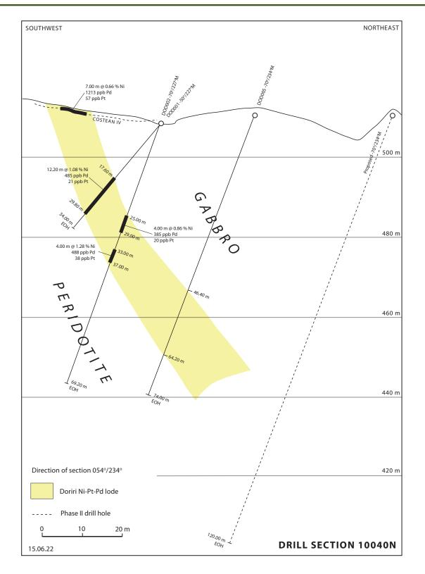
Drill section 10040N showing existing holes DOD001 and DOD002, completed in 2012, present hole DOD005 and a proposed hole
