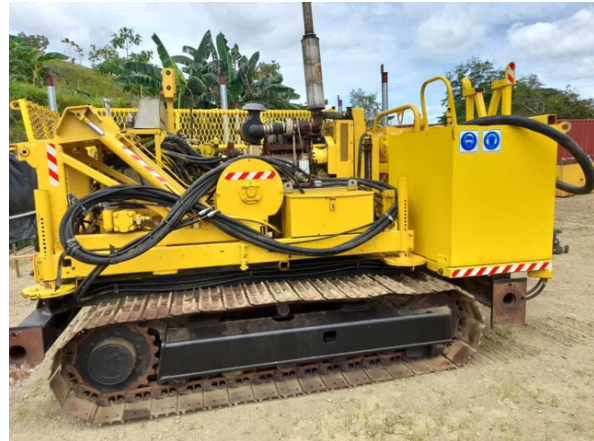
Figure 3: Omu drill pad prepared (left) and Golden Birch's newly acquired CS1000 Drill Rig to be used to drill holes up to approximately 500m in length (right).
